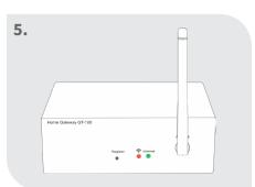
Both diodes light up permanently: Gateway active
